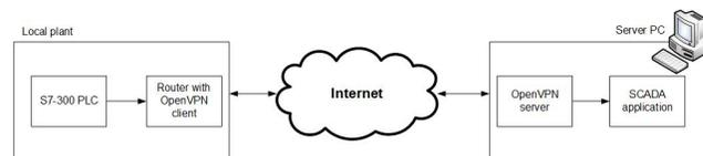
Fig. 2. Remote data acquisition and control using OpenVPN
