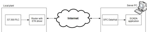
Fig. 3. Remote data acquisition and control using OPC tunneling
