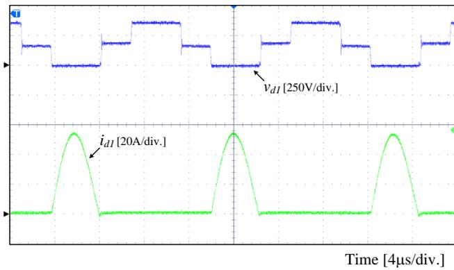
Fig. 10. Experimental results for the soft-switching technique on the output diode  $D_T$ .
