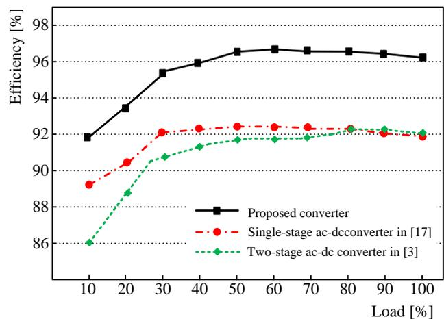
Fig. 13. Efficiency comparison according to the converter topology.
