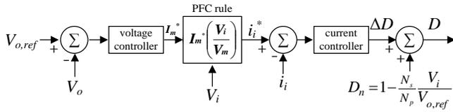
Fig. 6. Proposed control block diagram for the single-power-conversion.
