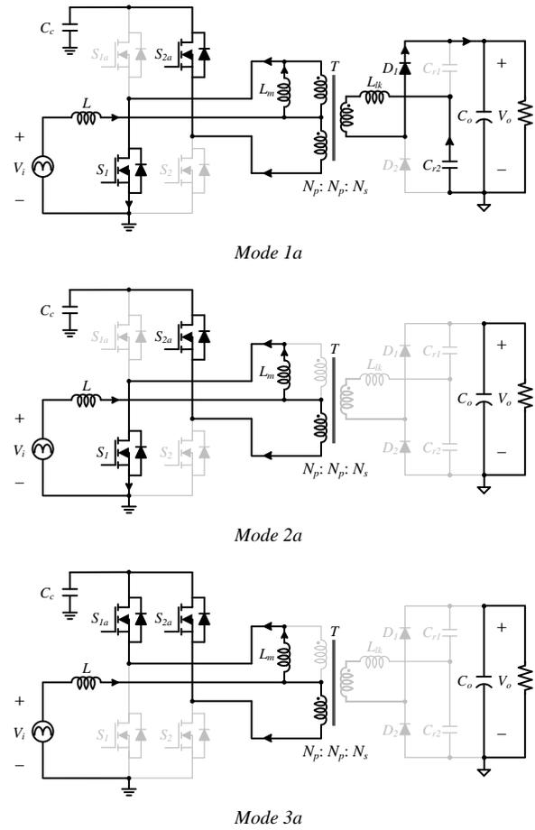
Fig. 3. Equivalent circuits of the proposed converter for  $D < 0.5$  during half switching period,  $T_s/2$ .
