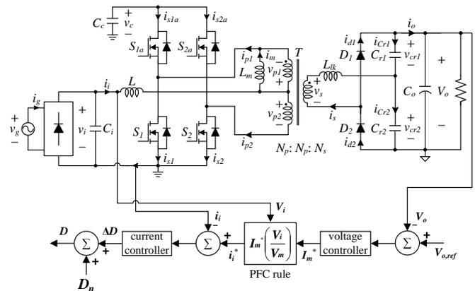
Fig. 1. Circuit configuration and control block diagram of the proposed converter.
