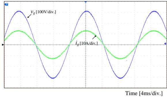
Fig. 8. Experimental waveforms for the grid voltage  $v_g$  and the grid current  $i_g$ .
