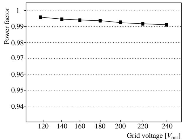
Fig. 12. Measured power factor according to the grid voltage level.
