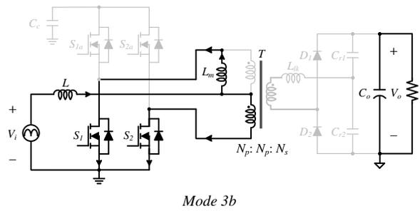
Fig. 5. Equivalent circuit of the proposed converter for  $D > 0.5$  in the overlapped region.
