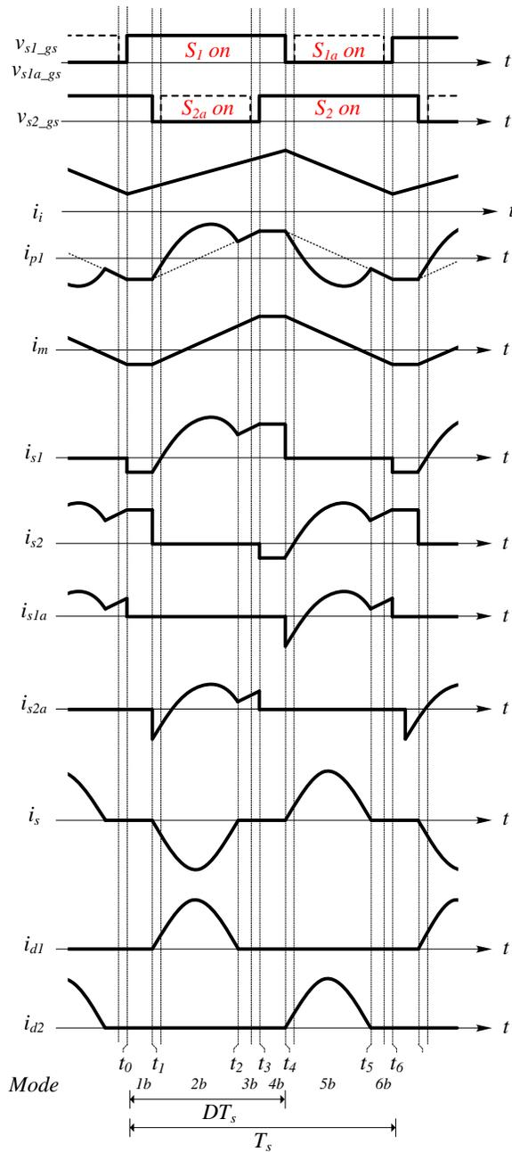
Fig. 4. Key waveforms of the proposed converter for  $D > 0.5$ .
