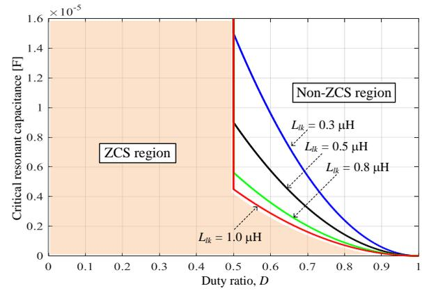
Fig. 7. ZCS region of the proposed converter according to circuit design.
