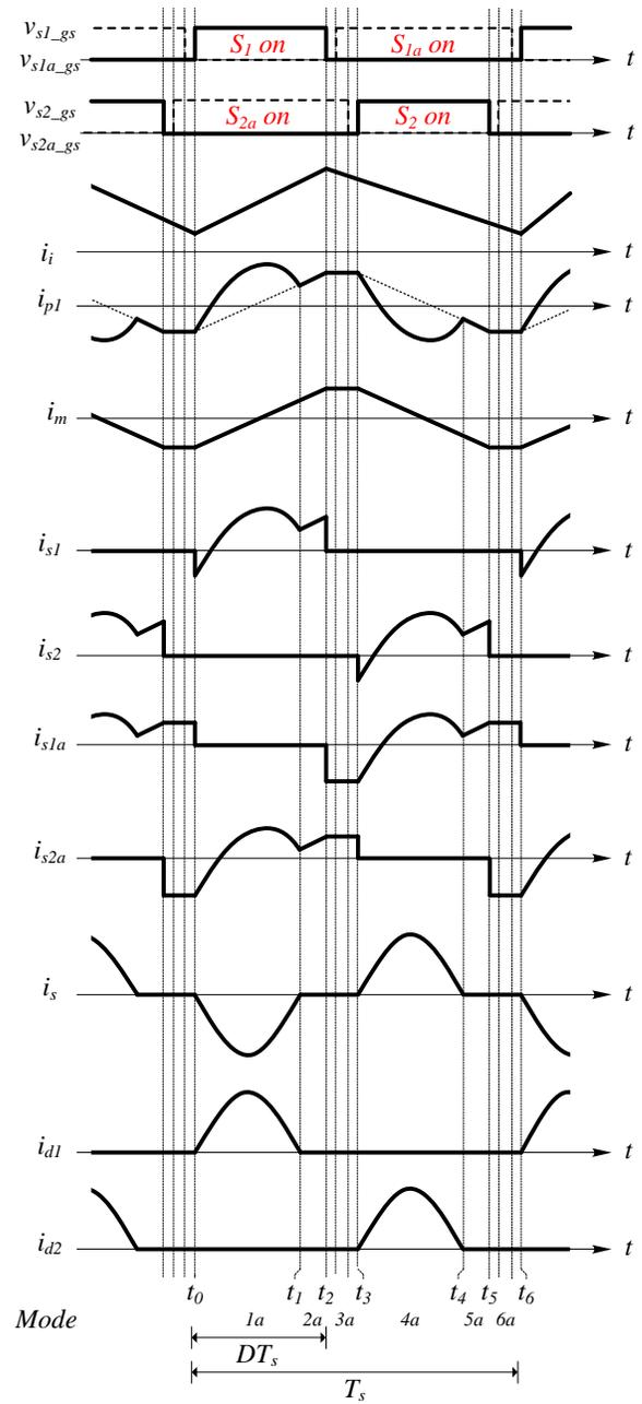
Fig. 2. Key waveforms of the proposed converter for  $D < 0.5$ .
