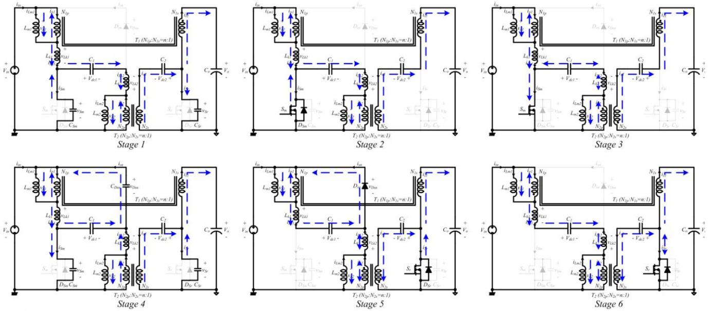
Fig. 5. Operating stages of the proposed converter.
