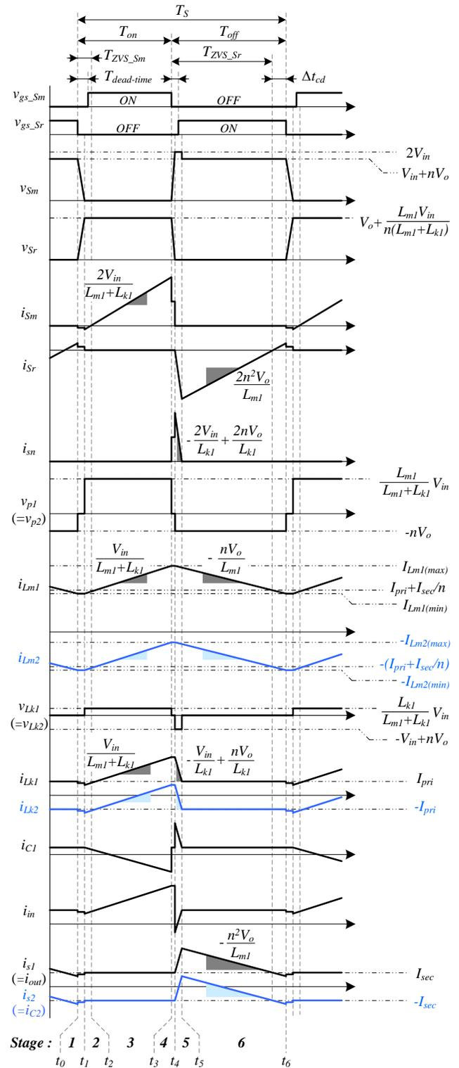
Fig. 4. Theoretical waveforms of the proposed converter.
