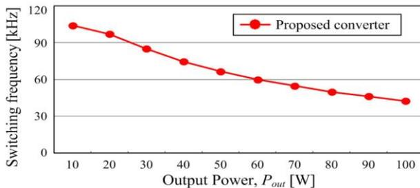
Fig. 14. Measured switching frequency of the proposed converter.
