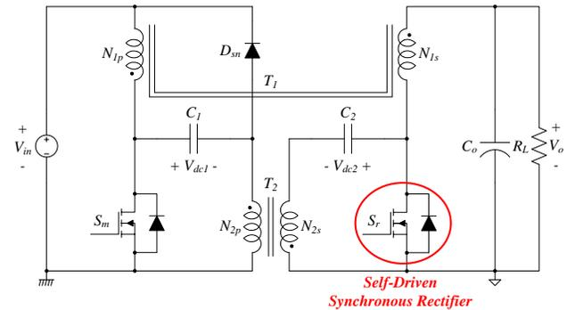
Fig. 2. Proposed converter with self-driven synchronous rectifier.
