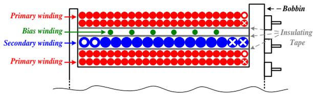
Fig. 10. Structure of the coupled inductor.
