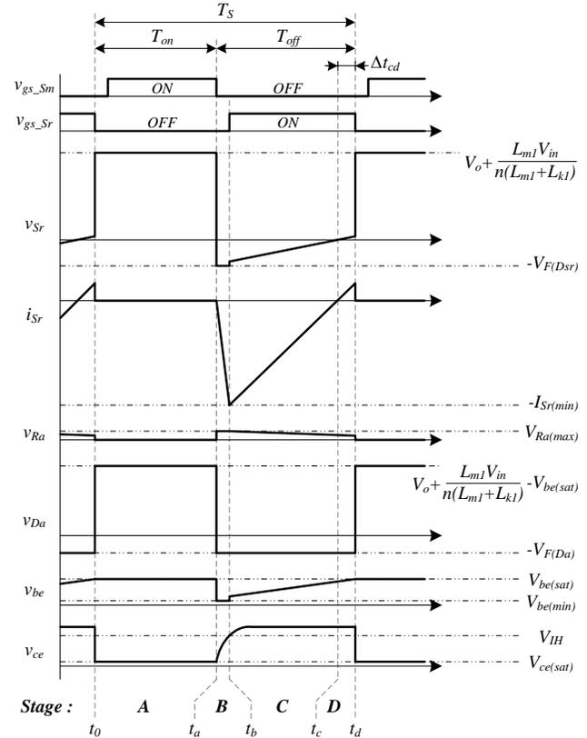
Fig. 7. Theoretical waveforms of the proposed SR driver.
