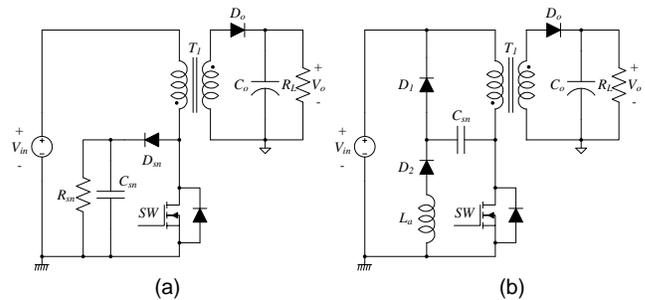
Fig. 1. Conventional flyback DC-DC converter : (a) with a RCD snubber, (b) with a LCD snubber.
