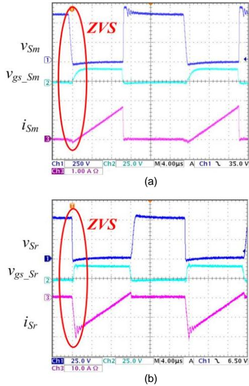
Fig. 12. ZVS operations of  $S_m$  and  $S_r$  at 100W: (a)  $v_{Sm}$ ,  $v_{gs\_Sm}$ ,  $i_{Sm}$  (b)  $v_{Sr}$ ,  $v_{gs\_Sr}$ ,  $i_{Sr}$ .
