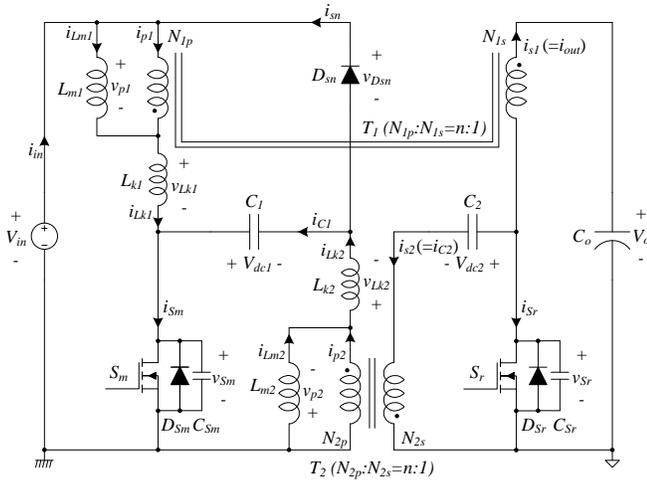
Fig. 3. Equivalent circuit of the proposed converter.
