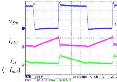
Fig. 11. Experimental waveforms of  $v_{Sm}$ ,  $i_{Lk1}$ ,  $i_{S1}(=i_{out})$  at  $P_o=100W$ .
