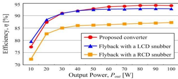
Fig. 13. Measured efficiencies of the proposed and conventional converters.
