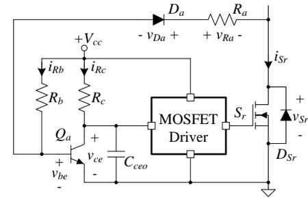
Fig. 6. Self-driven synchronous rectifier driver.
