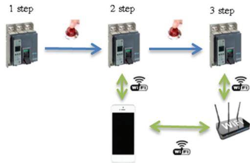
Fig. 3. Diagram of the steps of connection to Wi-Fi for programming.
