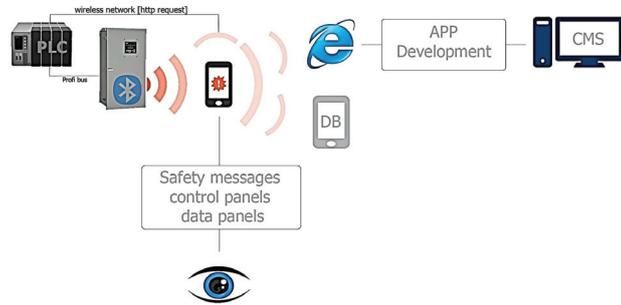
Fig. 6. Diagram explaining the using of beacons for controlling electrical apparatus.
