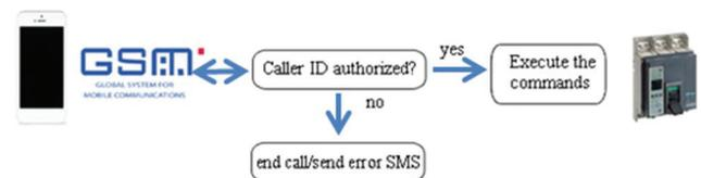
Fig. 1. Diagram of GSM based model operation.
