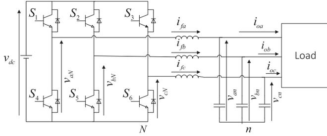
Fig. 1. Three-phase inverter with an LC filter.
