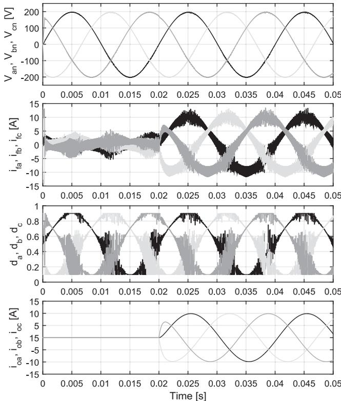
Fig. 3. Simulation results: Output voltages, filter currents, duty cycles, and load currents for inductive load.
