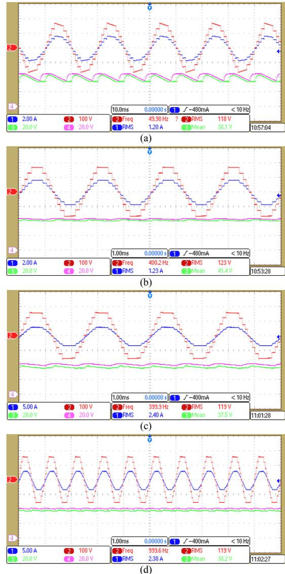
Fig. 4. Measurements of the 9-level SCMLI prototype (CH1:  $V_o$ ; CH2:  $i_o$ ; CH3:  $V_{c1}$ ; CH4:  $V_{c2}$ ); (a) driving a 100 $\Omega$ -1mH load at 50Hz; (b) 100 $\Omega$ -1mH load at 400Hz; (c) 50 $\Omega$ -1mH load at 400Hz; (d) 50 $\Omega$ -1mH load at 1kHz
