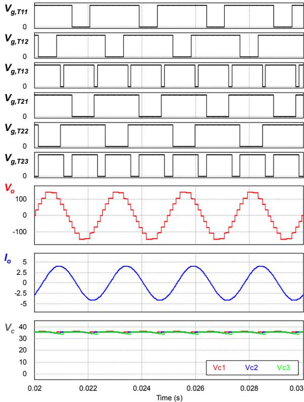
Fig. 3. Simulation result of a 9-level SCMLI; the gate driver signals for the 1<sup>st</sup> and 2<sup>nd</sup> SC units; the output voltage, current and the voltages of capacitors
