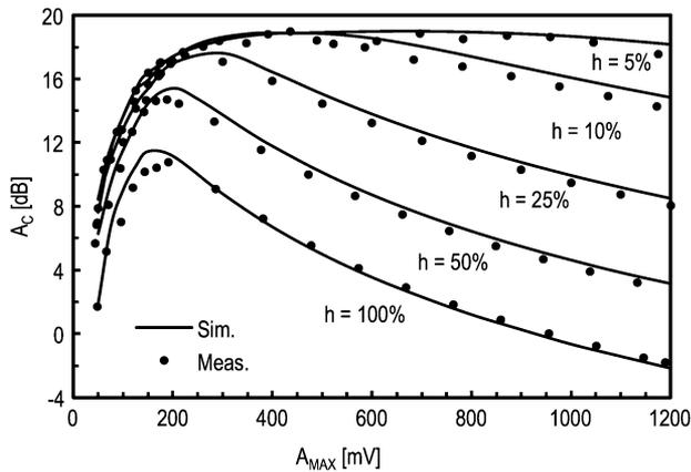
Fig. 6. Measured and simulated conversion gain as a function of  $A_{MAX}$ , for various modulation indexes.
