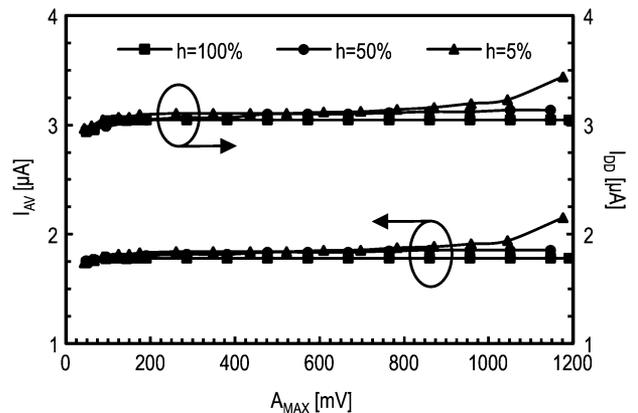
Fig. 9. Measured average current consumption of (a) the input pair ( $I_{AV}$ ) and (b) the whole ASK detector ( $I_{DD}$ ) for  $h$  values of 5%, 50%, and 100%.
