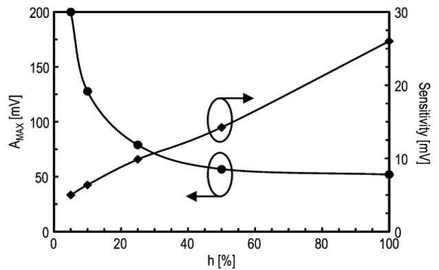
Fig. 8. Measured sensitivity of the proposed detector and corresponding  $A_{MAX}$  as a function of modulation index  $h$ .
