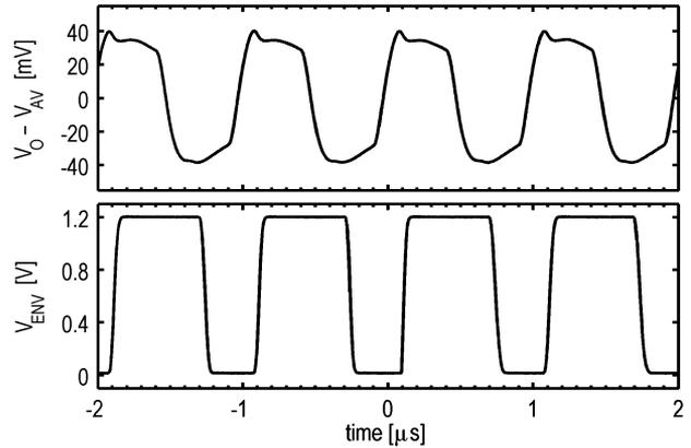
Fig. 7. Measured output waveforms at sensitivity ( $h = 5\%$  and  $A_{MAX} = 200$  mV).
