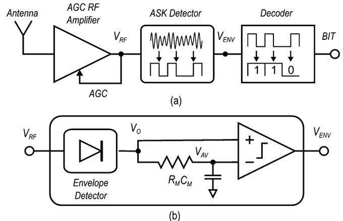
Fig. 1. Typical architecture of (a) an ASK receiver and (b) an ASK detector.
