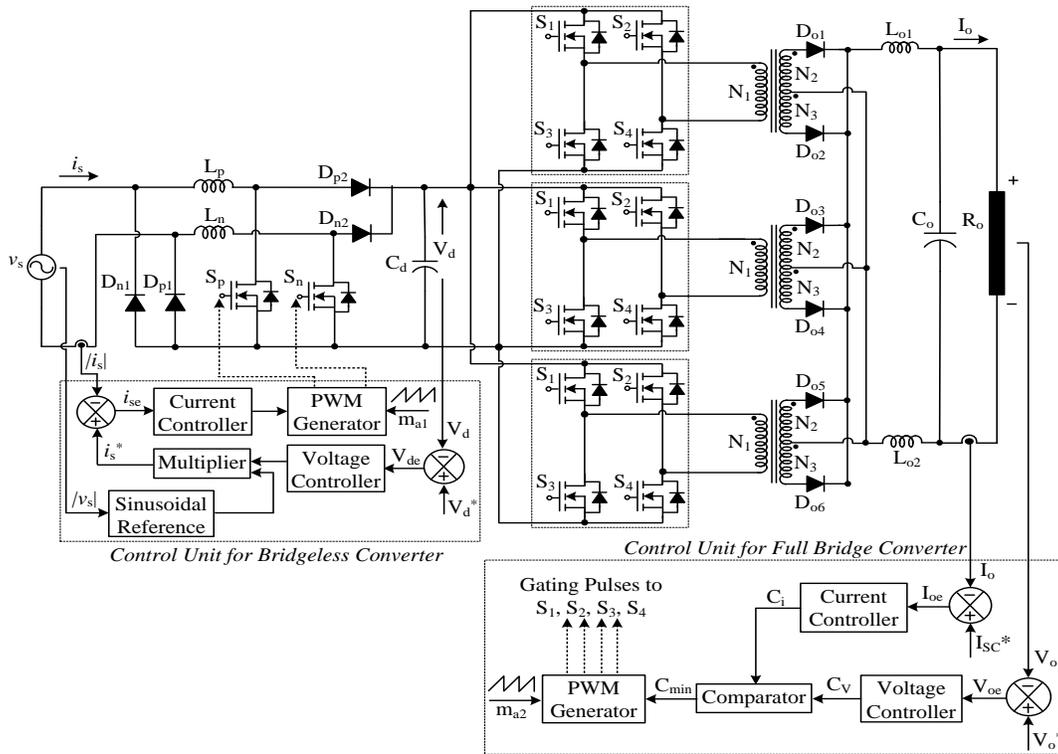
Fig.2. Schematic of BL boost converter and isolated FB converter based AWPS.
