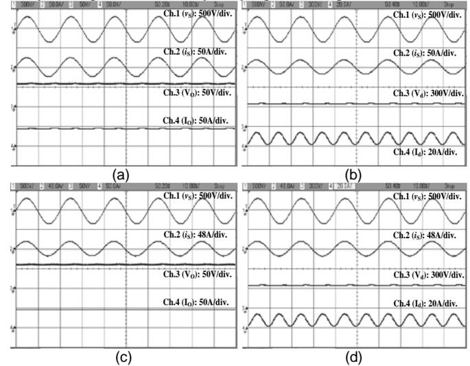
Fig.6. Test results under supply voltage variations. (a) Waveforms of  $v_s$ ,  $i_s$ ,  $V_o$  and  $I_o$  at rated load and at  $v_s = 183V$ ; (b) Waveforms of  $v_s$ ,  $i_s$ ,  $V_d$  and  $I_d$  at rated load and at  $v_s = 183V$ ; (c) Waveforms of  $v_s$ ,  $i_s$ ,  $V_o$  and  $I_o$  at rated load and at  $v_s = 256V$ ; (d) Waveforms of  $v_s$ ,  $i_s$ ,  $V_d$  and  $I_d$  at rated load and at  $v_s = 256V$ .
