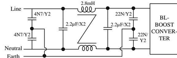
Fig. 11. EMI filter for the proposed BL-Boost converter based AWPS.
