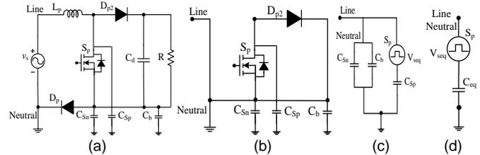
Fig. 10. Building of EMI model of proposed BL-Boost converter.
