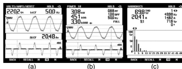
Fig.1. Recorded PQ indices of AWPS (with DBR) at rated load with supply voltage as 220V; (a) Input voltage and current; (b) Input power and PF; (c) Harmonic spectrum of input current.
