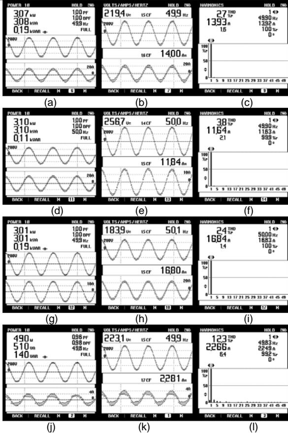
Fig.8. PQ indices of proposed BL boost converter based AWPS; (a)–(c) at rated load and  $v_s=220$  V, (d)–(f) at rated load and  $v_s=256$ V, (g)–(i) at rated load and  $v_s=183$ V (j)–(l) at light load and  $v_s=220$  V.
