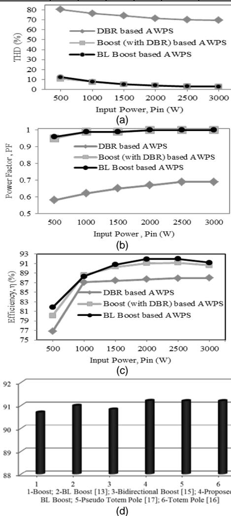
Fig.9. Comparative analysis of (a) THD of supply current (b) PF (c) efficiency for the conventional, boost (with DBR) and proposed BL boost converter based AWPS; (d) efficiency of different BL boost configurations.
