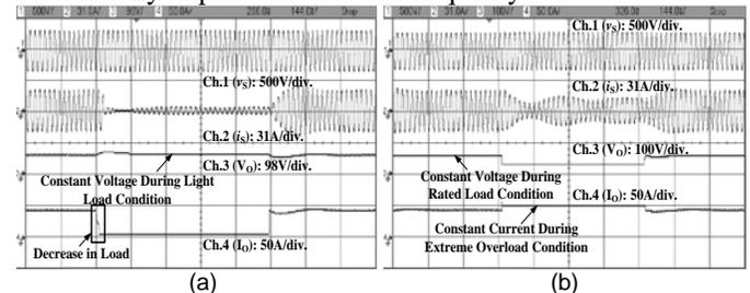
Fig.7. (a)  $v_s$ ,  $i_s$ ,  $V_o$  and  $I_o$  under light load condition; (b)  $v_s$ ,  $i_s$ ,  $V_o$  and  $I_o$  under overload condition.
