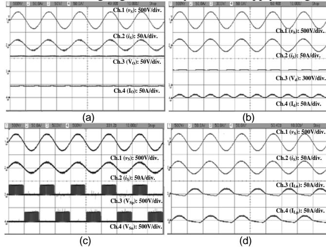
Fig.5. Steady state performance of proposed converter at rated load and 220V (rms) supply voltage. (a) Waveforms of  $v_s$ ,  $i_s$ ,  $V_o$  and  $I_o$ ; (b) Waveforms of  $v_s$ ,  $i_s$ ,  $V_d$  and  $I_d$ ; (c) Waveforms of BL converter switch voltage stress  $S_p$  and  $S_n$ ; (d) Waveforms of  $v_s$ ,  $i_s$ ,  $I_{Lp}$  and  $I_{Ln}$ .
