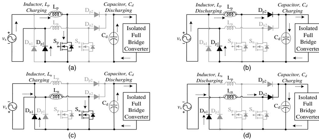
Fig. 3. Operation of the steady state BL boost converter during positive (a-b) and negative half-cycle (c-d) of the supply voltage. (a) Mode I and (b) Mode II during positive half cycle; (c) Mode I and (d) Mode II during negative half cycle
