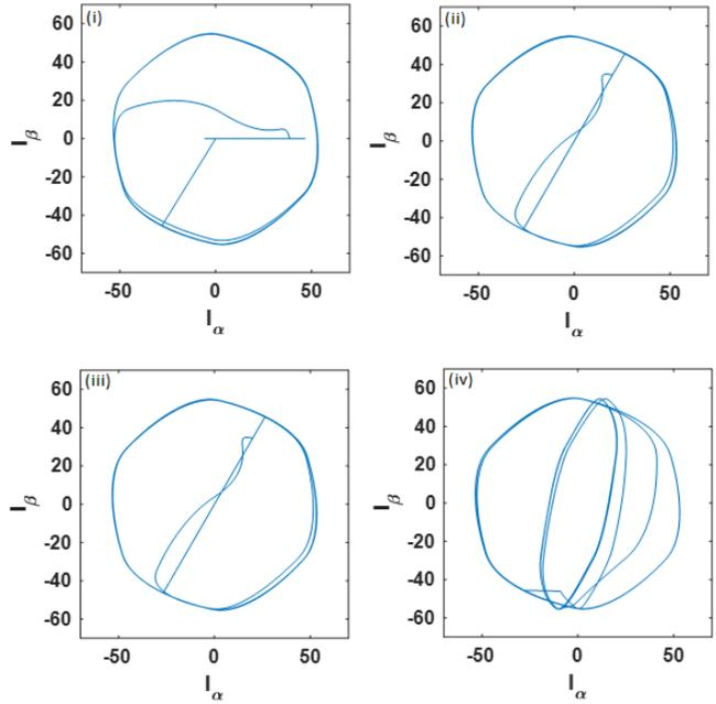
Fig. 7. Park trajectory in case of different faults as (a) LLL (b) LLG (c) LL and (d) LG
