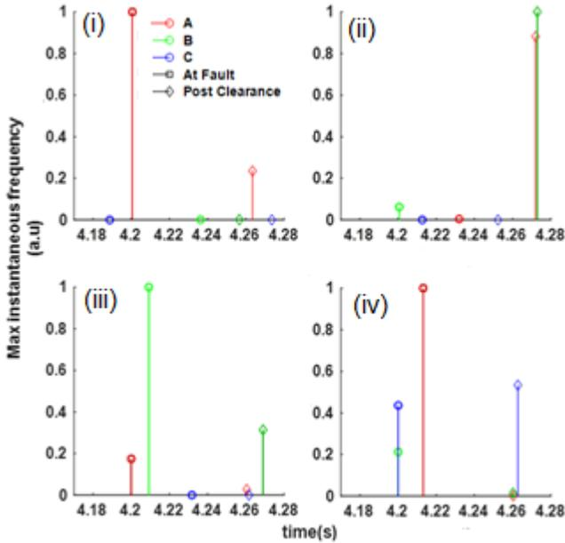
Fig. 9. Normalized maximum instantaneous frequency of different phase currents during (i) LG, (ii) LG, (iii) LLG, and (iv) LLL faults
