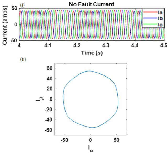
Fig. 3. (i) Load current and (ii) PVT for no fault current
