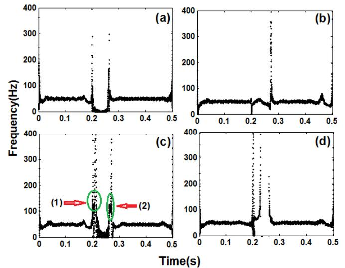
Fig. 8. Frequency-Time plot for different faults as in (a) LG (b) LL (c) LLG and (d) LLL
