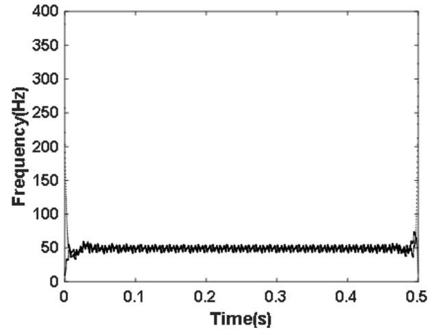
Fig. 4. Frequency-time plot in case of no fault obtained from HHT
