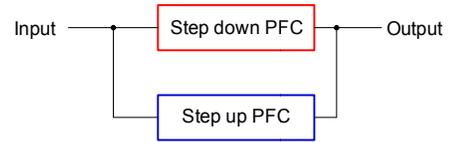
Fig. 3 Circuit diagram for hybrid PFC with parallel connection
