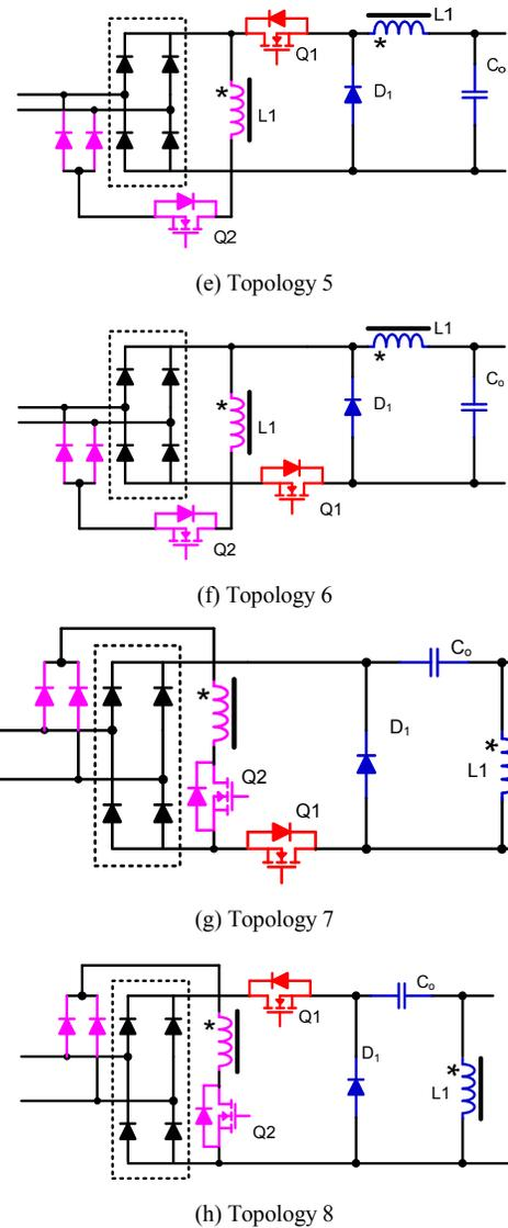
Fig. 6 Hybrid PFC with parallel connection – share the output block
