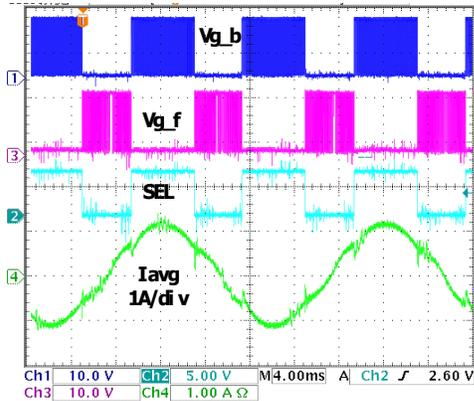
Fig. 10 Waveforms @Vin=90V ( $V_{g\_b}$  ( $V_{gs}$  for Q1),  $V_{g\_f}$  ( $V_{gs}$  for S2), SEL (mode selection),  $I_{avg}$  (average input current))
