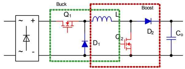
(b) Four-switch Buck-Boost converter
