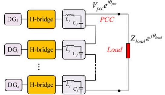
Fig. 1. Structure of islanded cascaded-type microgrid.
