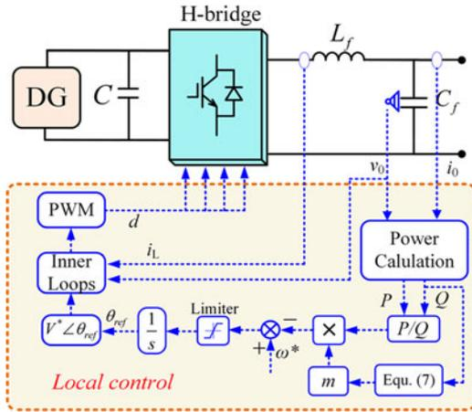
Fig. 2. The local control diagram of the  $i$ -th DG.
