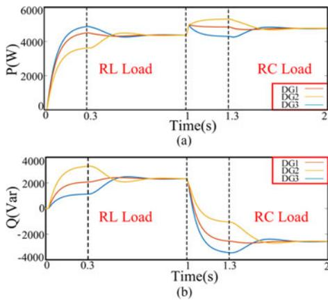
Fig. 3. Simulation results of case I. (a) Active power. (b) Reactive power.
