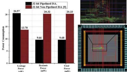
Fig. 4: Comparison plot of leakage, dynamic and total power consumed by 32-bit pipelined and non-pipelined ISA, when implemented in 90 nm-CMOS process and operated at 400 MHz clock frequency and chip layout of proposed 32-bit pipelined ISA with core area of  $5111 \mu\text{m}^2$  when implemented in UMC 90 nm-CMOS technology node.
