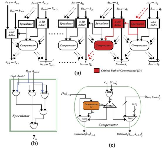
Fig. 1: (a) Basic block diagram of  $n$ -bit conventional inexact-speculation adder (ISA). (b) Gate-level circuit representation of speculator block. (c) Digital architecture of compensator block.
