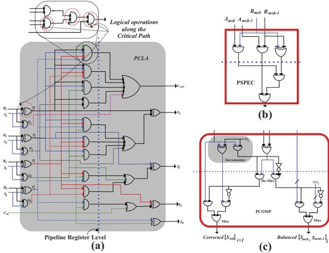
Fig. 3: Gate-level circuit of (a) Four-bit pipelined-carry look-ahead adder (PCLA) (b) Pipelined speculator (PSPEC) (c) Pipelined compensator (PCOMP) used in the proposed ISA VLSI architecture.
