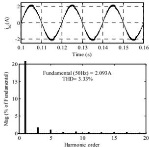
Fig. 4b Input current and its harmonic spectrum at full load condition
