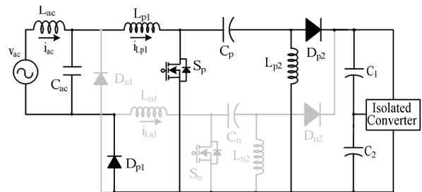
Fig. 2 Operation of PFC converter when the input voltage is positive
