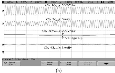
Fig. 11 (a) Recorded waveforms of  $v_{ac}$ ,  $i_{ac}$ ,  $V_{PFC}$  and  $I_{PFC}$  during ac input voltage variation
