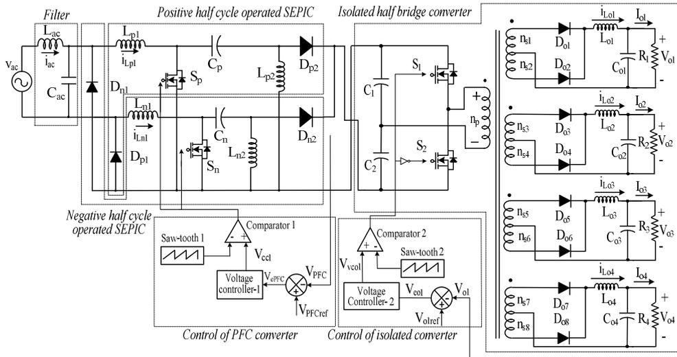
Fig. 1 Schematic diagram of PFC converter based SMPS
