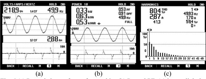
Fig. 6 (a) Recorded waveform of  $v_{ac}$  and  $i_{ac}$ , (b)  $P_{ac}$  and PF, (c)  $I_{THD}$  at light load condition
