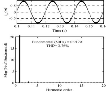
Fig. 5b Input current and its harmonic spectrum at light load condition
