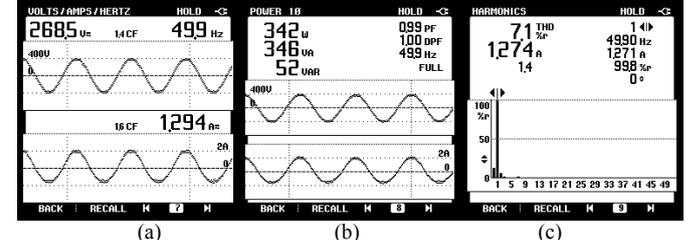
Fig. 9 (a) Recorded waveforms of  $v_{ac}$  and  $i_{ac}$ , (b)  $P_{ac}$  and PF, (c)  $I_{THD}$  at 270V
