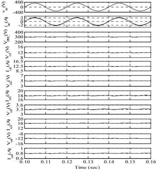
Fig.4a Performance of the computer power supply at rated condition
