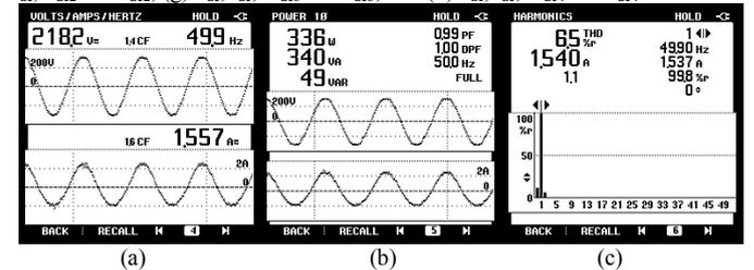
Fig. 8 (a) Recorded waveforms of  $v_{ac}$  and  $i_{ac}$ , (b)  $P_{ac}$  and PF, (c)  $I_{THD}$  at full load
