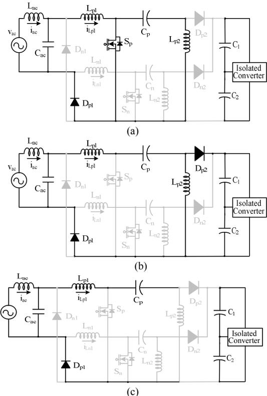
Fig. 3 Operating modes of bridgeless PFC converter when the input voltage is positive
