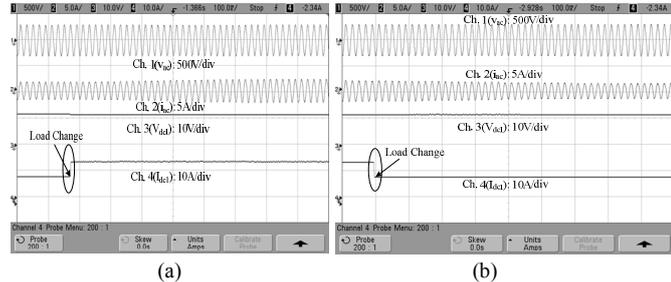
Fig. 13 (a) Recorded waveform of load increase in  $I_{dc1}$  (b) Recorded waveform of load decrease in  $I_{dc1}$
