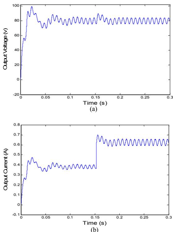
Fig.10. The output waveforms for load changes from 210 $\Omega$  to 128 $\Omega$ . (a) The output voltage. (b) The output current.
