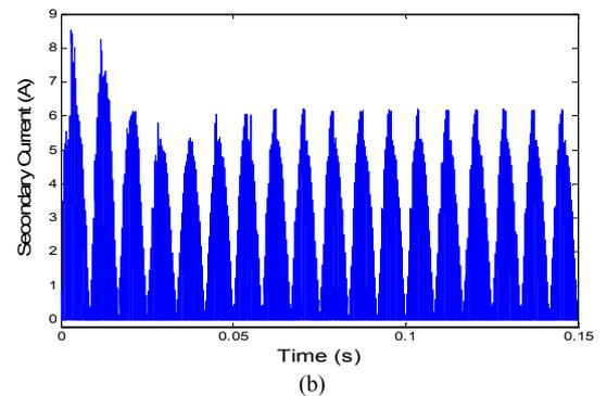
Fig.7. The waveforms of current of transformer. (a) The primary current. (b) The secondary current.
