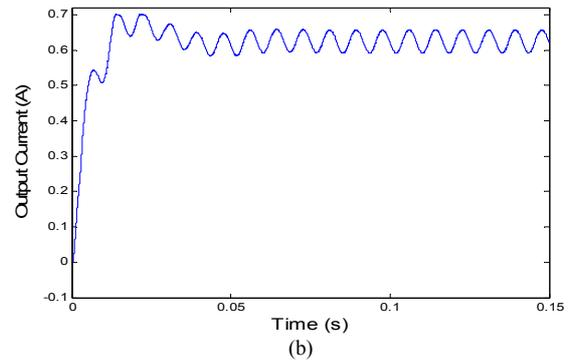
Fig.6. The output waveforms for 128  $\Omega$  output load. (a) The output voltage. (b) The output current.
