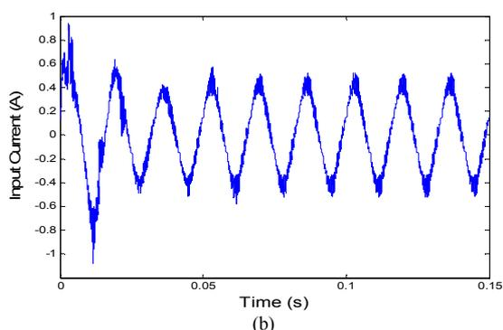
Fig.8. The input waveforms for 128  $\Omega$  output load. (a) The input voltage. (b) The input current.
