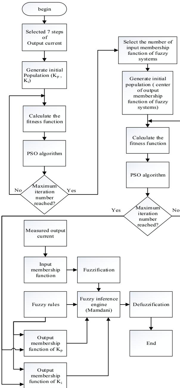
Fig.5. Flowchart of the proposed control method.
