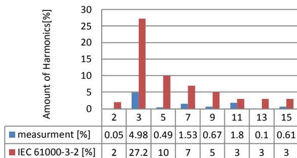
Fig.9. The spectrum of the input current.
