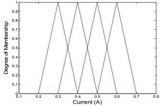
Fig.4. The input functions of fuzzy algorithm.
