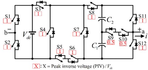
Fig. 2. The proposed single-stage switched-capacitor module (S<sup>3</sup>CM) topology for cascaded MLI.
