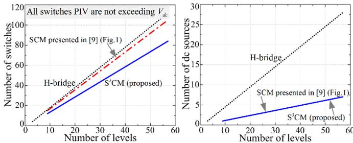
Fig. 4. Comparative analysis for cascaded MLI using the proposed S<sup>3</sup>CM, SCM [9] (Fig. 1) and H-bridge.
