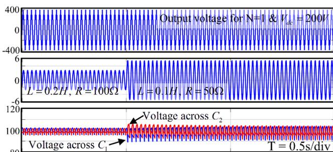
Fig. 8. Simulated waveforms for step load change.
