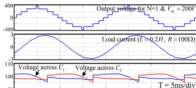
Fig. 6. Simulated steady-state waveforms for single S<sup>3</sup>CM (9-level).
