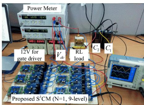
Fig. 10. Experimental prototype.
