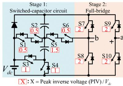
Fig. 1. Switched-capacitor module (SCM) topology presented in [9].
