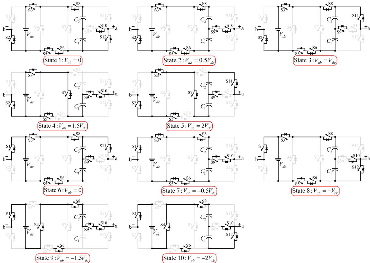
Fig. 3. Switching states of the proposed S<sup>3</sup>CM topology.
