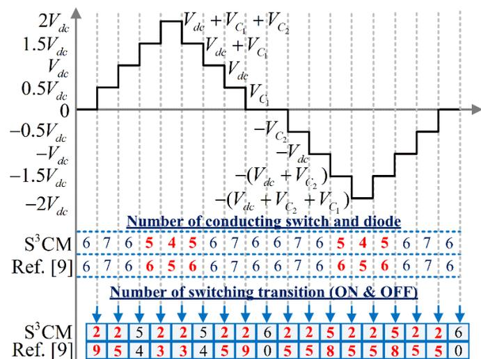
Fig. 5. Comparisons between the proposed S<sup>3</sup>CM and the SCM in [9].
